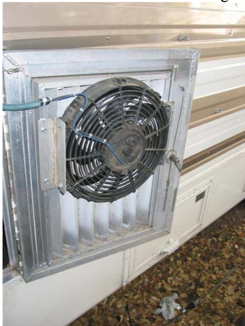
Fan mounted on the inside of the grill
